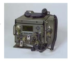
**Qual, Low-Power System.** A two transceiver, low power system should be used when co-site performance is required at the 10W level, as two Spectre V transceivers are stacked in a single mount. The system allows for simultaneous transmission and reception on the same vehicle.
